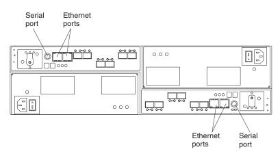
Figure 51. Ethernet and serial port locations on DS5020
